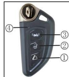
turned off. At this time, the power lock knob cannot be turned. If you need to turn the knob, press the power lock knob downward to verify the validity of the key. After verification passes the indicator will be turned on for 5 seconds (in blue), the turn signal light will flash once and the buzzer will sound once, and the power lock knob can be turned within the 5 seconds.
