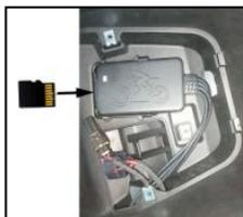
push the TF card forward and remove it after popping out. It is necessary to format the new TF card once via the computer first and its format should be FAT32.
