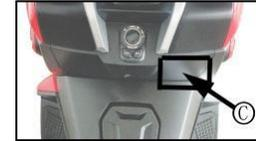
the electronic remote-control key is out of power, put the remote-control key close to the antenna position (about 4-5cm), and the keyless controller (PKE) can sense the remote-control key and unlock the power lock.
