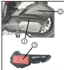
It must be confirmed that the air filter element is firmly installed in the original position and is properly sealed.
