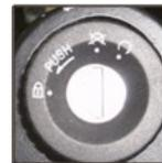
○ Mark.. The key turns to the marked position "○", the power is on, the engine can be started, and the key cannot be taken out;
