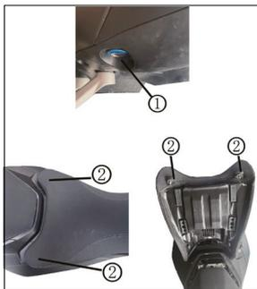
Remove the screws ② on both sides of the driver's seat cushion, pull it backwards and then lift it upwards to remove the driver's seat cushion.
