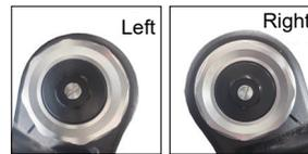
Factory adjustment is 2 turns (use a slotted screwdriver to adjust the adjusting bolt clockwise
