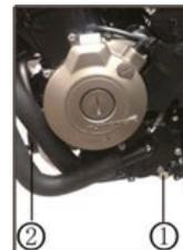
①. Use the special tool for removing the engine oil filter to clamp the engine oil filter and rotate it counterclockwise to remove the engine oil filter to be replaced.
