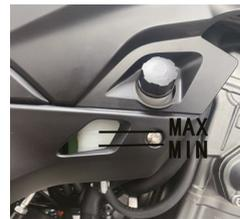
When the new vehicle leaves the factory, the coolant has been installed, and attention should be paid to the inspection of the coolant level in the expansion pot during maintenance.
