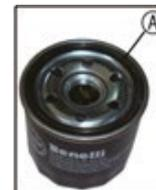
③. Use a new oil filter of the same type and apply a layer of lubricating oil on the O-ring (A).
