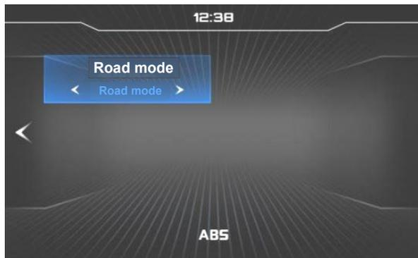
4.1.2 When the “Off-road” is set, “ABS” will be shown, then Road mode is switched in white font after pressing and releasing the button . Press the button , the ABS function will be shown with blue underline; Press and release the button to show the ABS function in blue; Press and release the button and to select the ABS function: Enable or Disable.
