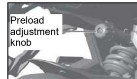
change the rebound speed of the shock absorber. The damping force adjusting nut will make a "click" sound every time it is adjusted to one gear. It has been marked when leaving the factory, and customers are advised not to adjust it by themselves. The preload value adjustment button is provided at the left side of the upper of the shock absorber. Turn it clockwise to increase, and turn counterclockwise to reduce with the limit distance of 10mm. Its factory state is one clockwise turn.
