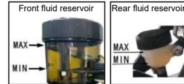
injected into the brake hose and the liquid level decreases accordingly. The front fluid reservoir is installed above the right handle of the vehicle. If the liquid level is lower than the mark MIN of the lower limit scale line of the fluid reservoir, the specified brake fluid shall be added as appropriate; The rear fluid reservoir is installed in the middle of the right
