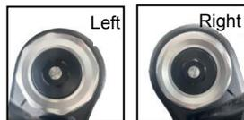
The force increases and the restoring damping force decreases for counterclockwise rotation (S direction). Adjust the left and right shock absorbers to the same damping force level.
