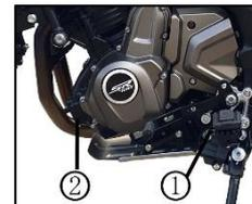
remove the oil drain bolt ①, completely drain the engine oil in the tank, reinstall the oil drain bolt with a torque of 20 ~ 25 N. M, and replace the engine oil filter ② according to the following steps:
