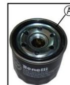
③. Use a new oil filter of the same type and apply a layer of lubricating oil on the O-ring ①.
