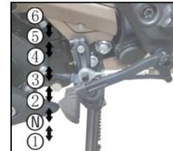
between the low gear and the second gear. From the neutral position, step down the shift lever to engage the low gear; every time the shift lever is lifted up by the toe, the next high gear is shifted; every time the shift lever is stepped on by the toe, the next low gear is shifted.
